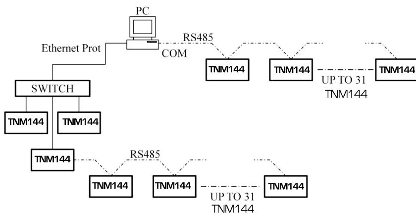
— TCP\IP ETHERNET (Shielded & Grounded)
