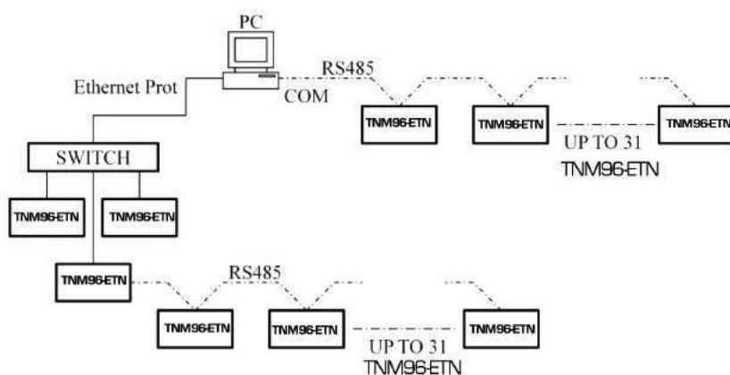
— TCP/IP ETHERNET (Shielded & Grounded)
